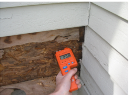
Excessive moisture readings due to improper construction methods
